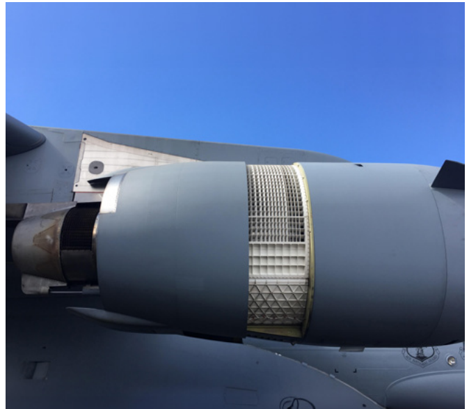
Figure 3. C-17 wing mounted F117 nacelle with thrust reverser deployed, showing cascades for providing reverse flow on upper half of the nacelle only.
