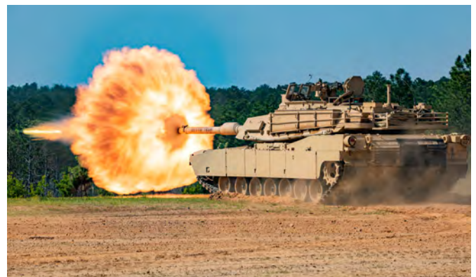
Figure 2. Multi-fueled AGT1500 powered M1A2 Abrams Tank, firing its 120 mm cannon. Tank hull is 26.02 ft (7.93 m) long and 12 ft (3.66 m) wide.
