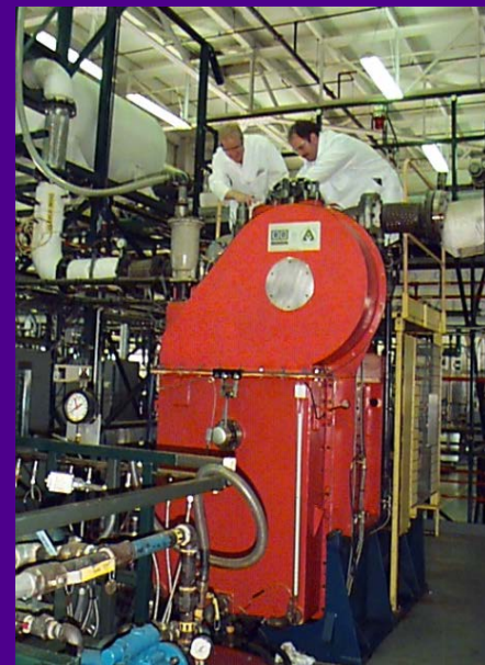
4-cycle Progress Rail H Engine at Argonne (16.6 L)
