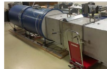
Airflow bench setup for measuring system impedance for components and servers and characterizing system performance when utilizing Air cooling .
