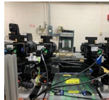
LaVision Tomographic PIV with PLIF capabilities for Immersion cooling studies. Other equipment: 2U SPIC & 2PIC tanks.
