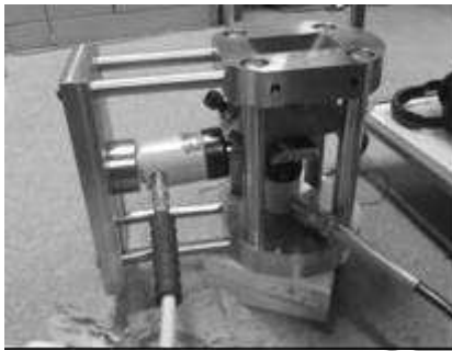
Figure 3. Photograph of the loading frame, showing the two hydraulic cylinders for applying normal and lateral loads.
