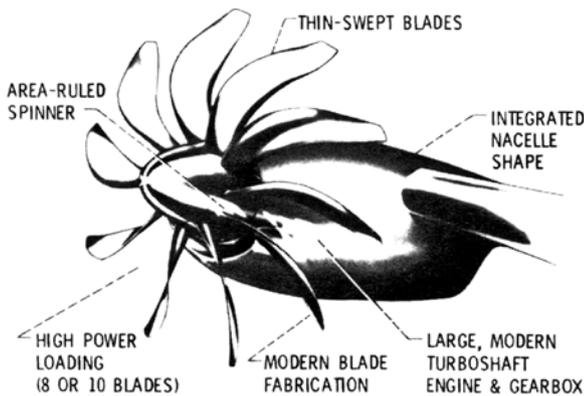
Figure 3. NASA 1980 high speed turboprop propulsion system. [4]
