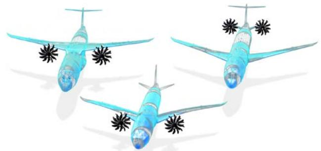
Figure 2. Possible RISE engine mounting positions on single-aisle airframes.
