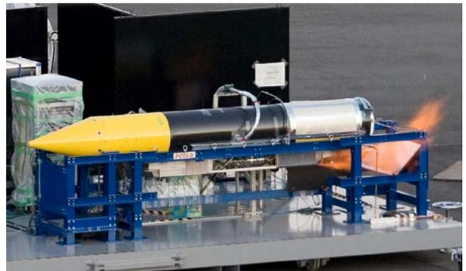
Figure 2. Sea Level Static Experiment of PCTJ.
