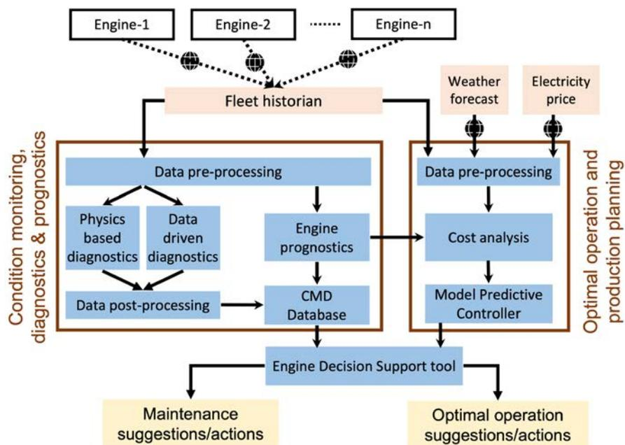
Figure 2. Framework for micro gas turbine fleet monitoring, diagnostics, and production planning.<sup>[4]</sup>
