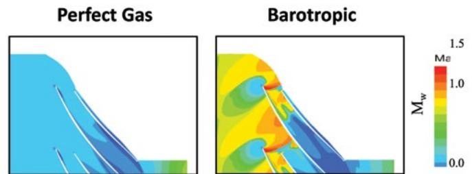
**Figure 4.** Comparison of relative tip Mach number fields obtained with the perfect-gas and barotropic model for three spanwise sections.
