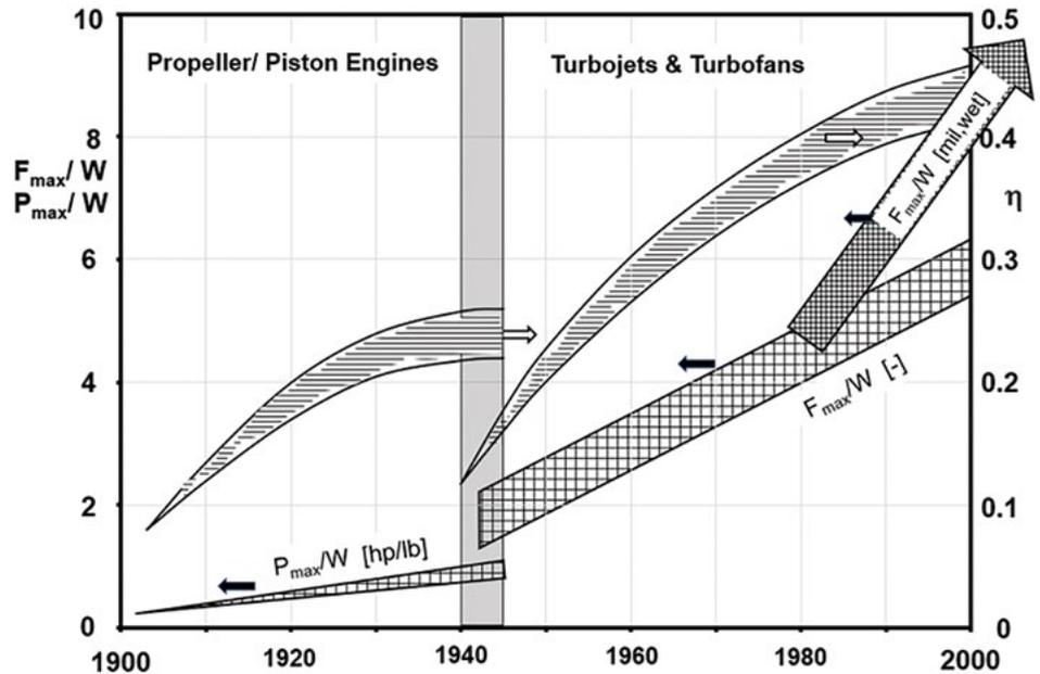
**Figure 2.** Aero propulsion systems from 1900 to 2000. Trends of power-to-weight ratio,  $P_{max}/W$  [hp/lb] for propeller/piston engines; thrust-to-weight ratio,  $F_{max}/W$  [lb/lb] for turbojets/turbofans, and overall engine efficiency,  $\eta$ .<sup>[2]</sup>
