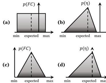
Figure 2 Probability distributions for (a) flow capacity at performance deterioration; (b) isentropic efficiency at performance deterioration; (c) flow capacity at production scatter; (d) isentropic efficiency at production scatter
