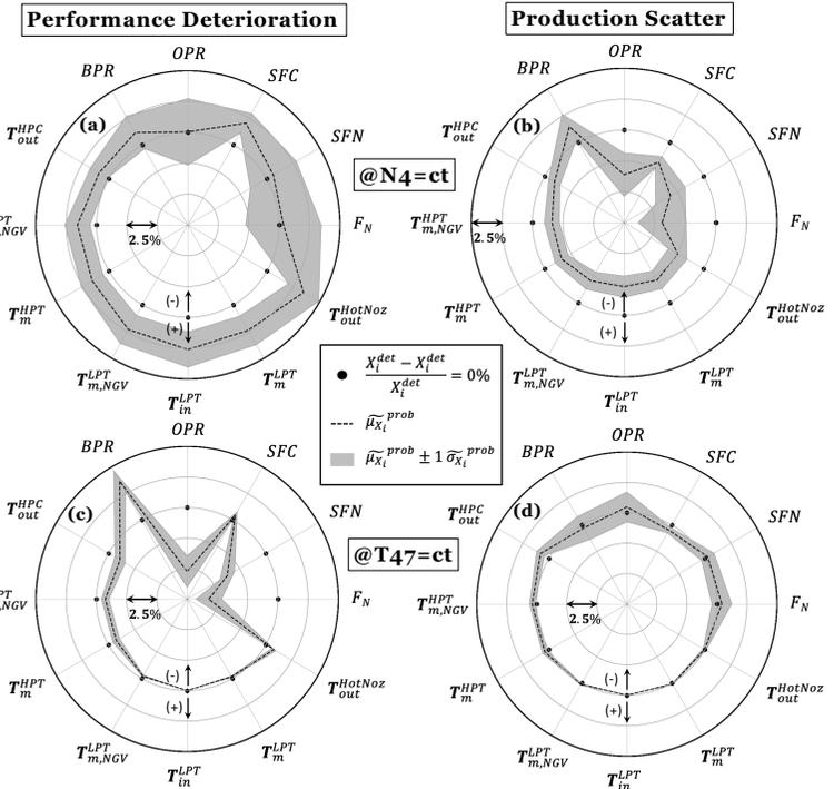
Figure 3 Probabilistic engine design properties when estimating: (a) Performance deterioration at constant N4; (b) Production scatter at constant N4; (c) Performance deterioration at constant T47 and (d) Production scatter at constant T47
