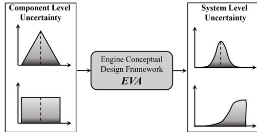
Figure 1 Flowchart of the probabilistic engine design
